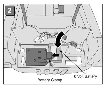
While pushing the battery clamp, place a Power Wheels®
